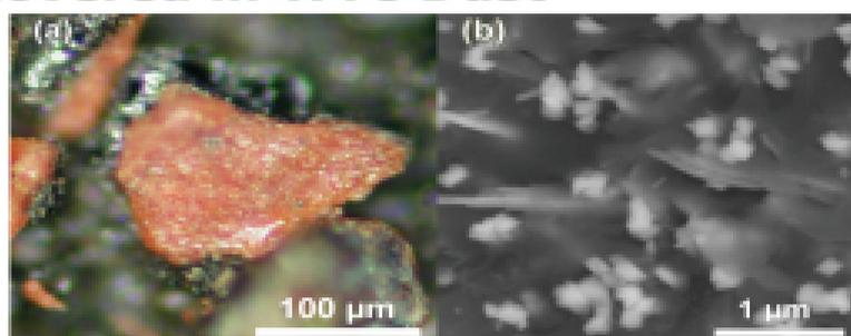
Highly energetic red/gray chip discovered in the WTC dust at optical magnification (a) and 50,000X electron microscope magnification (b). The latter image shows consistently sized iron oxide particles approximately 100 nm across and 40 nm-thick wafers of aluminum embedded in a carbon-rich matrix
